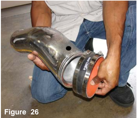
Figure 26 Press the 5 1/2" hose over the end of the intake. Use two power bands and tighten the clamp over the cast intake for now.
