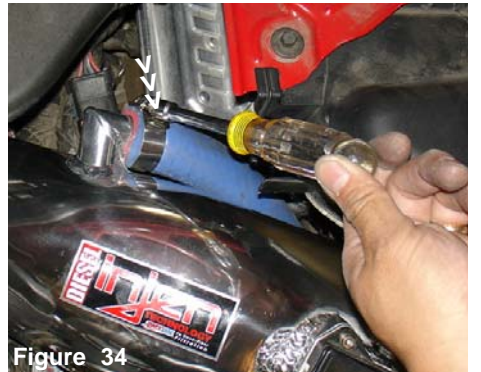
Figure 34 The clamp on the air recirculating breather hose is tightened with a nutdriver.
