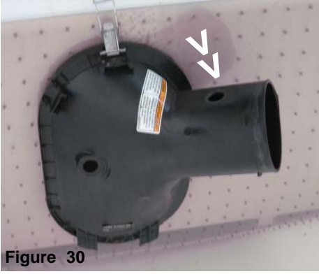
Figure 30 The stock grommet is removed from the air box cleaner.
