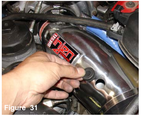
Figure 31 The stock grommet is pressed into the cast air intake as shown above.
