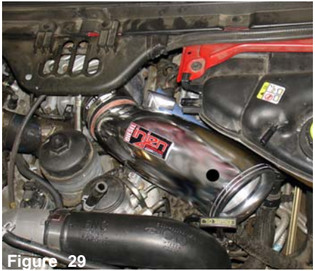
Figure 29 The 5 1/2" straight hose is now installed over the cast intake.
