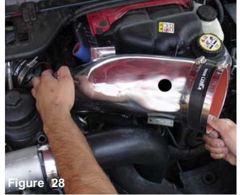
Figure 28 The assembled cast intake is lowered into the engine compartment. the smaller end is pressed into the turbo hose
