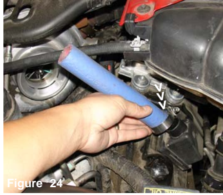
Figure 24 The 25mm hose is pressed over the air recirculator port.
