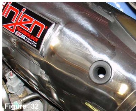
Figure 32 The stock grommet is pressed into the 3/4" hole as shown above.
