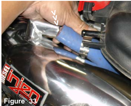
Figure 33 The 25mm air recirculating hose is pressed over the 90 degree intake port.
