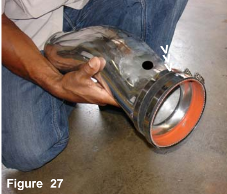
Figure 27 The straight hose is pressed over the cast intake end and the clamp is tightened on the intake side.
